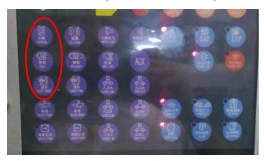
2. Copy all the datas and settings to papers in the controller or take photos of these pages because all the parameters would be resetted and you would have records for reference (remember there are some settings in the hiden pages by pressing CANCEL+MOLD/SATA and press CANCEL+CURSOR DOWN), password is 654321;
